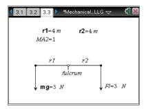
Q11. Derive a formula for the mechanical advantage of a first-class lever in terms of the lengths of the two arms of the lever, **r1** and **r2**. (Hint: The torques created by both forces, effort and resistance, are equal.)
