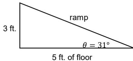
$$\begin{aligned} \sin 31^\circ &= \frac{3}{\text{ramp}} \quad \text{or} \quad \cos 31^\circ = \frac{5}{\text{ramp}} \\ \text{ramp} &= \frac{3}{\sin 31^\circ} \quad \text{ramp} = \frac{5}{\cos 31^\circ} \\ \text{ramp} &\approx 5.82 \text{ ft.} \quad \text{ramp} \approx 5.83 \text{ ft.} \end{aligned}$$
